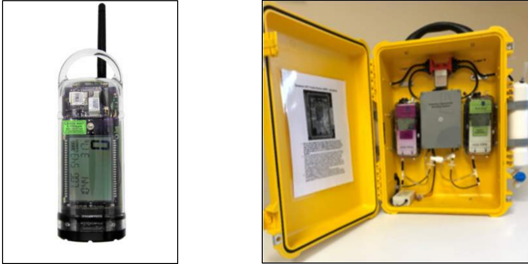
Figure 3.2 Acrulog™ Standalone Monitor (left) & LRSS Assembly with Acrulog™ monitors (right).
